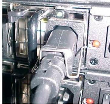
3. Pull the power cord out of the failed power supply and set it aside.
