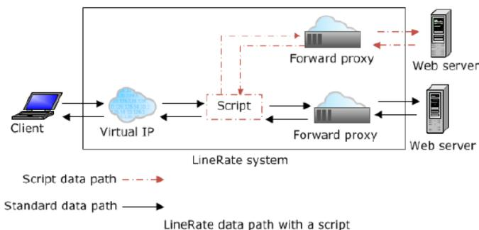
In this example, the script "intercepts" the request just before it reaches the forward proxy. The script sends the request to a different forward proxy from the standard data path, based on what the script
