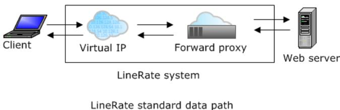
In the standard data path, the request comes in from the client, goes through the virtual IP, gets passed to a forward proxy, and finally to the web server. The response follows the same path back to the client.
