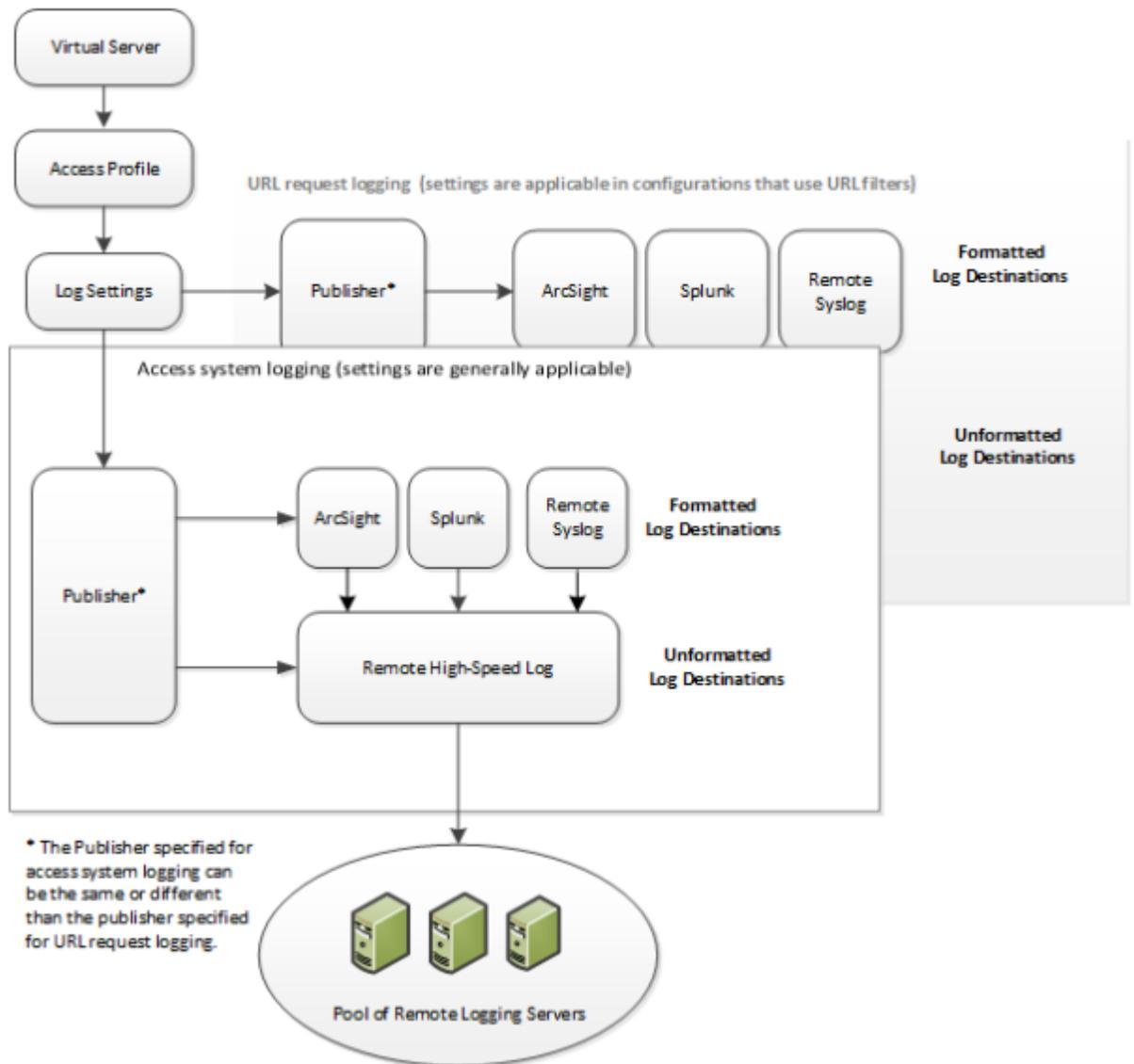
Figure 5: Association of remote high-speed logging configuration objects
