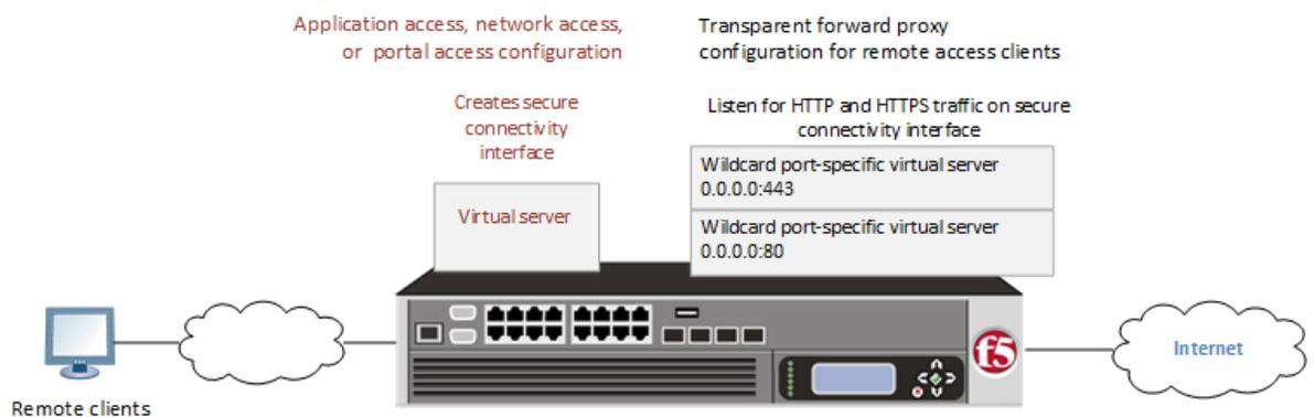
Figure 2: Transparent forward proxy for remote access
