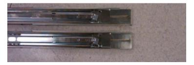
7. Install the slide rails on the inside rail of the equipment rack. Insert the thumb screws provided in the top and bottom holes by screwing them through the cabinet rails and into the slide-bracket threaded inserts. (Leave the middle hole open.)
