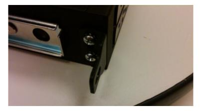
4. Assemble the front slide-rail mount brackets (the short ones) to slide-cabinet members, as shown below, using the wing nuts provided.
