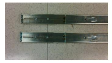
5. To determine the location of the rear-rail mount brackets, measure the inside surface of the front rail to the inside surface of the back rail of the equipment rack where the chassis will be installed.
