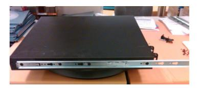
3. Install the two rail-locking brackets (found in the Accessory Kit bubble bag) using the 6-32 screws provided. (These are the 4 smaller screws. Save the 2 larger screws to lock the chassis into the equipment rack in step 14.) The following figure shows an installed locking bracket.
