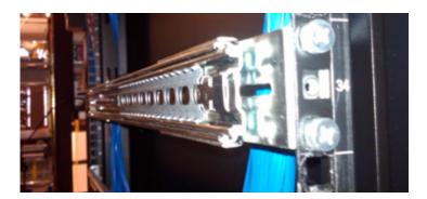
8. Repeat Step 7 to secure the slide rail to the rear equipment rack rail.
