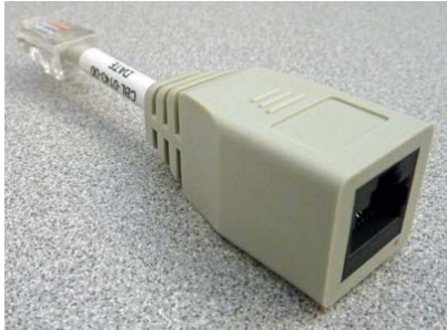
Figure 11: The RJ45F to RJ45M rolled serial (pass-through) adapter
