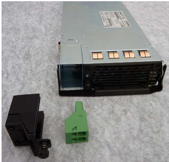
Figure 13: VIPRION 2400 DC power supply, lock assembly, and plug
