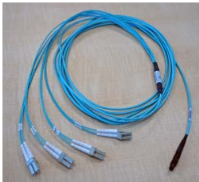
Figure 7: An example of a 40 GbE QSFP+ breakout cable
