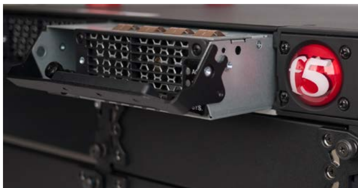
Figure 12: A power supply partially removed from the platform
